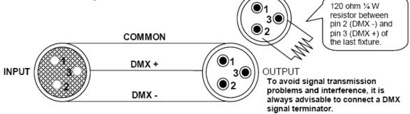
Do not allow contact between the common and the fixture's chassis ground. Grounding the common can cause a ground loop, and your fixture may perform erratically. Test the cables with an ohmmeter to verify correct polarity and to make sure the pins are not grounded or shorted to each other.
