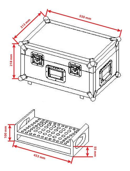
**Case Stacking for 48x conical truss connectors**
