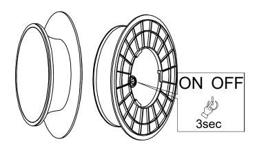
The lamp can also been controlled without Smart device: Press the power button once to switch mode between:
