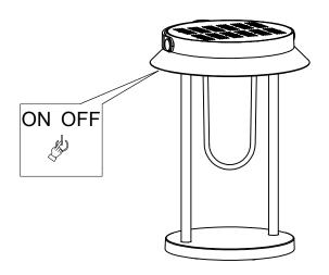
The lamp can also been controlled without Smart device: Press the power button once to switch mode between:
