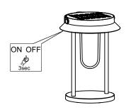
3. Press the Power button to turn on the lamp (if the lamp has been paired with another device before, please reset the lamp, see page 10)
