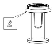
Hold power button for 3 seconds, the lamp will flash in blue, lamp has now been reset and automatically turn to pairing mode
