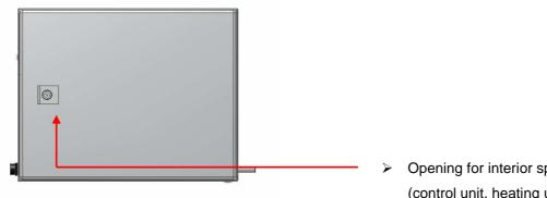
Opening for interior space (control unit, heating unit, fluidpumps)
