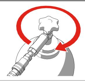
Move the manual CO<sub>2</sub> valve in OPEN position to release the pressure from the system.
