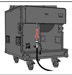
Disconnect the CO<sub>2</sub> hose from the CO<sub>2</sub> bottle-to-hose connector on the CO<sub>2</sub> cylinder.
