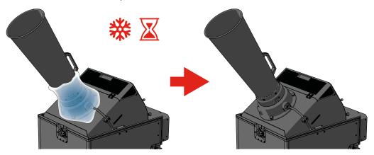
9 In case you have set the hopper under an angle: Position the hopper back in horizontal position (position 1).
