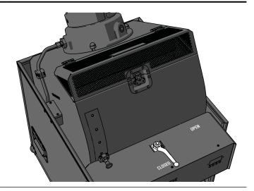
**2** Close the connected CO<sub>2</sub> cylinder.
