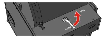
**4** Move the manual CO<sub>2</sub> valve back in CLOSED position.
