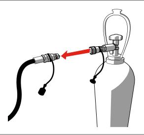
6 Remove the CO₂ bottle-to-hose connector from the cylinder.
