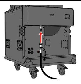
**12** Connect a  $CO_2$  bottle-to-hose connector to a  $CO_2$  cylinder.
