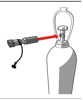
13 Connect the CO<sub>2</sub> hose to the CO<sub>2</sub> bottleto-hose connector on the CO<sub>2</sub> cylinder.
