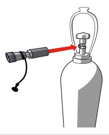
8 Connect the CO<sub>2</sub> hose to the CO<sub>2</sub> bottleto-hose connector on the new CO<sub>2</sub> cylinder.
