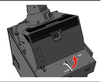
Disconnect the CO<sub>2</sub> hose from the CO<sub>2</sub> quick connector.
