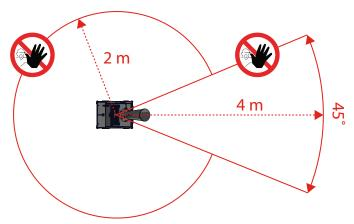
Place the MAGICFX® STADIUMBLASTER in its final position and set the brakes.
