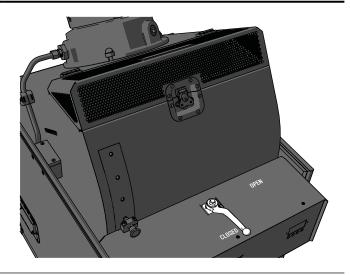
11 Connect the CO<sub>2</sub> hose to the CO<sub>2</sub> quick connector.
