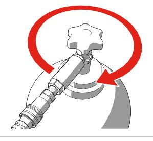
4 Move the manual CO<sub>2</sub> valve in OPEN position to release the pressure from the system.
