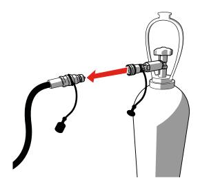
**7** Remove the CO<sub>2</sub> bottle-to-hose connector from the cylinder.
