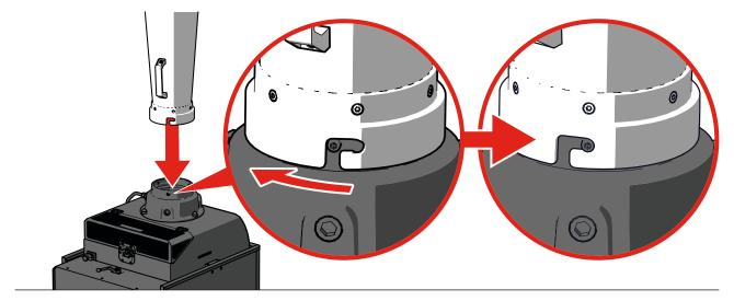
**6** Secure the woofer with the safety steel.
