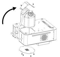
Fix the removable plate to the opposite side and fit the tank with the bottle lock again.
