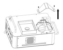
Remove the screws and the bottle lock to take out the tank.
