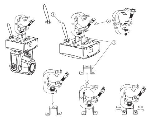
Screw one clamp via a M12 screw and nut to the included bracket. Attach the bracket using the included screws to the bottom of the Inno Pocket Spot. Attach the eyehole screw to the bottom of the base and pull the safety-cable through the screw and over the trussing system or a safe fixation spot. Insert the end in the carabine and tighten the safety screw.
