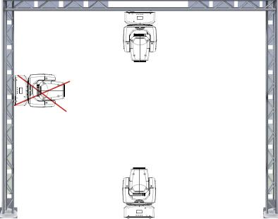
The Inno Pocket Spot is fully operational in two different mounting positions, hanging upside-down from a ceiling or set on a fat level surface. To avoid internal damage to the unit, never mount the unit on its side as illustrated above. Be sure this fxture is kept at least 0.5m away from any fammable materials (decoration etc.). Always use and install the supplied safety cable as a safety measure to prevent accidental damage and/or injury in the event the clamp fails (see next page).
