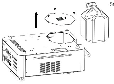
Step 2: Turn the machine upside down and remove the screws to release the plate.
