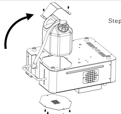
Step 3:Fix the removable plate to the opposite side and fit the tank with the bottle lock again.
