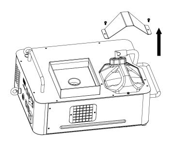
Step 1:Remove the screws and the bottle lock to take out the tank.
