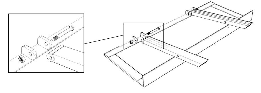
2. install the braces with bolts M10x95 at the right direction as drawing
