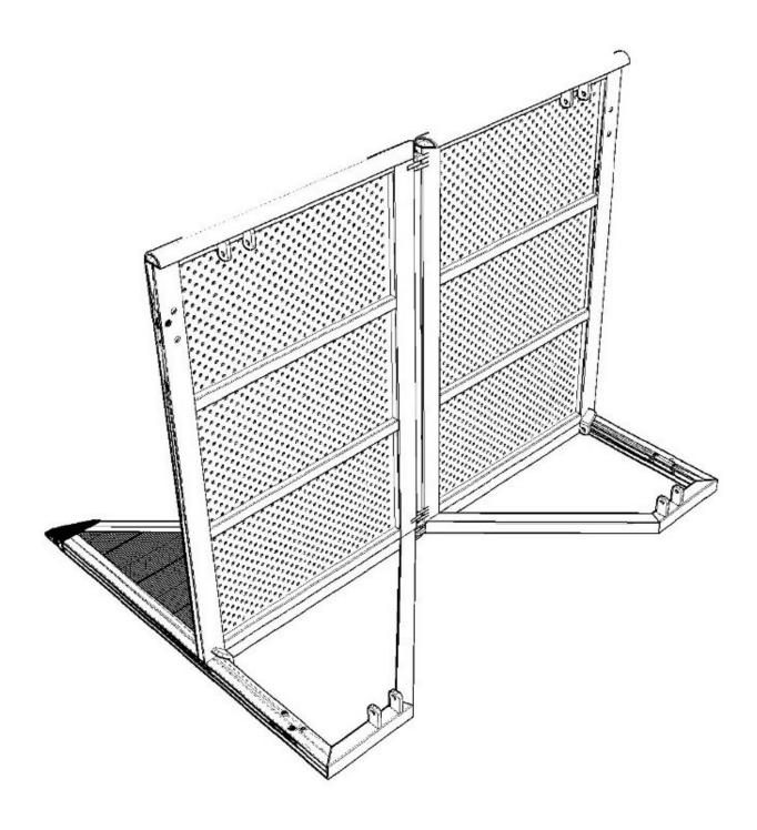
4. Make the installed vertical plate upright to the installed base plate, as drawing
