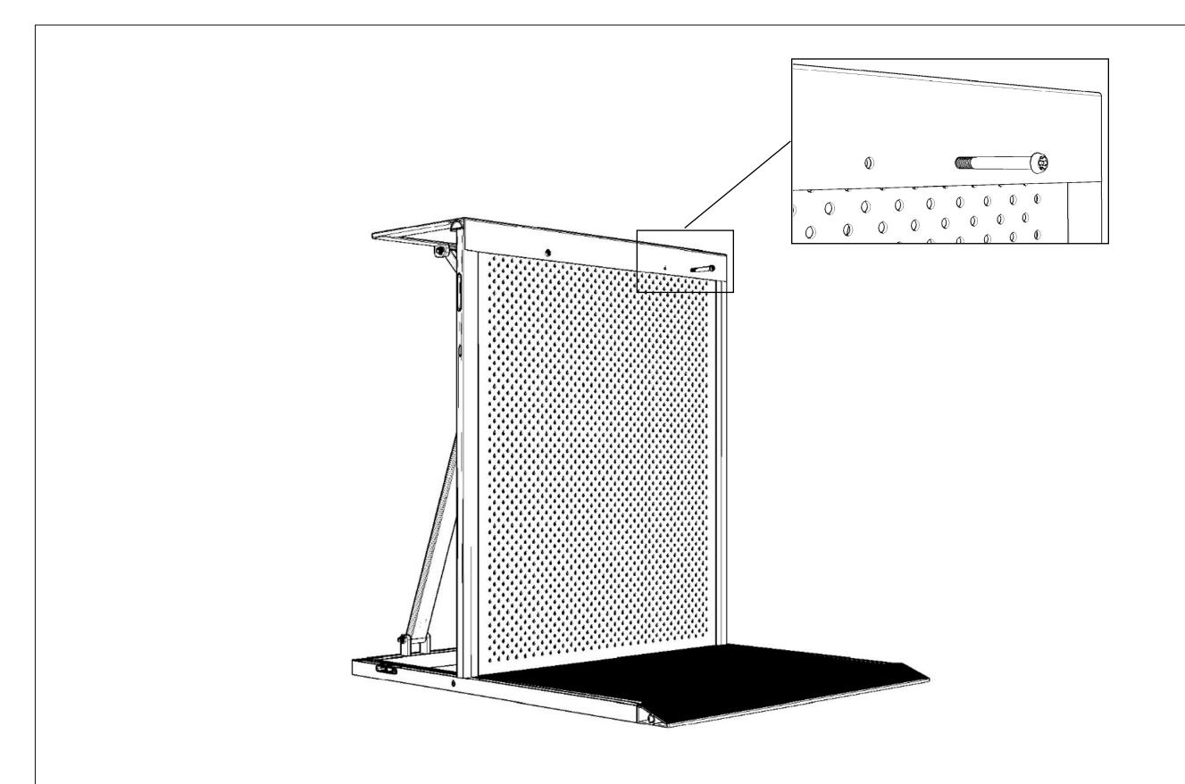
5. Use bolts M8 to connect the barrier table and the General Type at the front top as drawing
