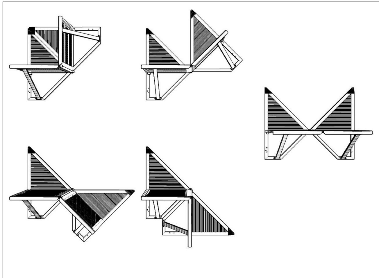
6. Adjust the angle from 90 degree to 270 degree as needed ( Please refer to General Type Manual for usage )
