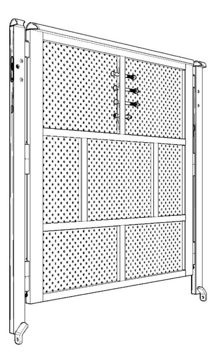
1. Rotate the two end profiles and make the vertical plate slide up and down
