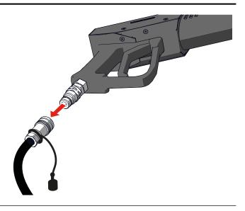
Disconnect the CO<sub>2</sub> hose from the CO<sub>2</sub> bottle-to-hose connector on the CO<sub>2</sub> cylinder.
