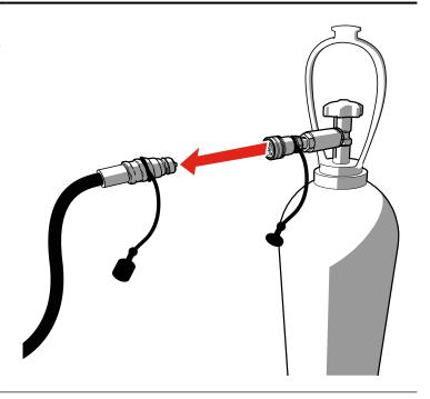
7 Remove the CO₂ bottle-to-hose connector from the cylinder.
