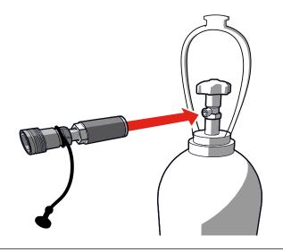
4 Connect the CO<sub>2</sub> hose to the CO<sub>2</sub> bottleto-hose connector on the CO<sub>2</sub> cylinder.
