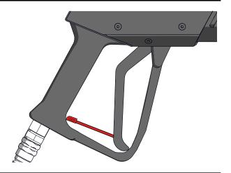
5 Disconnect the CO<sub>2</sub> hose from the CO<sub>2</sub> quick connector on the pistol.
